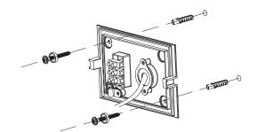
Fix the base on the wall and make the wires through the hole of the base.
