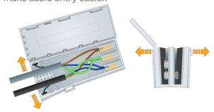
7. Try to keep cables of a similar size together in the same slot and simply push them into the slot as far as they will go. Once all the cables are installed, firmly squeeze the gripper end of the box together and snap shut the lid so that it is held securely by the 3 locking tabs.
